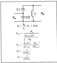
Figure 5. Capacitive-tap matching network.
