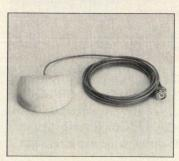
ver. These electrodes are printed on both sides of an extremely high dielectric constant ceramic substrate. Beneath this antenna element is the LNA utilizing proprietary GaAs FETs developed by Murata Erie. A 14 dB return loss is guaranteed over the full 15 MHz bandwidth of this 1575.42 MHz (L1 band) antenna. It boasts a 90 degree Kelvin noise temperature and minimum power at band center of 20 dB.
