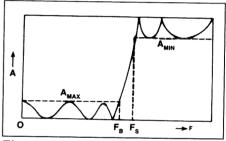
Figure 1. Elliptic filter response and some defining parameters.
