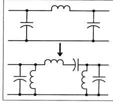
Figure 1. Lowpass filter transformed to bandpass filter.
