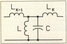
Figure 8. Inductively coupled resonator.
