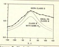
Figure 9. Variation of efficiency with series load reactance.
