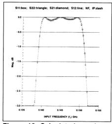
Figure 13. Calculated passband response of example filter.
