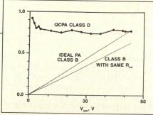
Figure 8. Variation of efficiency with output voltage.
