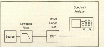
Figure 5. Harmonic distortion of a signal source can be improved by installing a lowpass filter.
