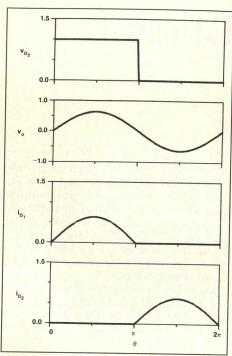
Figure 2. Waveforms of ideal complementary class-D PA.
