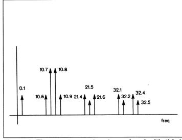
Figure 2. The spectrum a two-tone signal with thirdorder distortion products.
