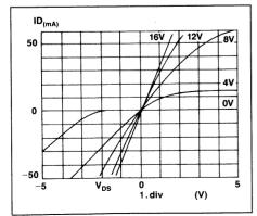
Figure 2. Typical MOSFET V-I characteristics.
