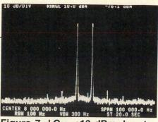
Figure 7. LO = +13 dBm, Input = +8.5 dBm, V BIAS = 3.4 V.
