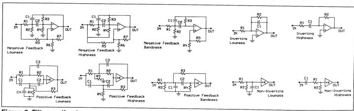
Figure 2. Filter section types.
