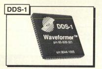
Clock .....up to 25 MHz Spurs @ 20 MHz ck .. <-60 dBc after the DAC Digital modulation ...... amplitude, phase, freq Dimensions ...... 1" x 1", or eval board
