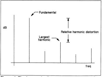
Figure 4. The harmonic distortion of a signal is often specified y stating the largest harmonic relative to the fundamental.
