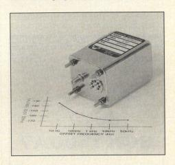
$2\times10^{-8}$ /year in a  $2\times2\times2.75$  inch package. Temperature stability is  $\pm5\times10^{-10}$  over 0 to +50 degrees C and  $\pm5\times10^{-9}$  over -55 to +75 degrees C. Frequencies are available to 75 MHz. Price is \$850 at 100 pcs., with delivery in 14 to 16 weeks.
