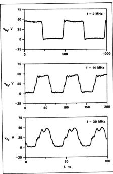
Figure 5. Drain voltage waveforms.
