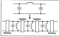
Figure 2. Lowpass filter transformed to coupled parallel resonators.
