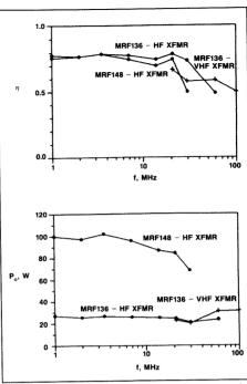
Figure 6. Output power and efficiency.
