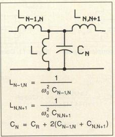
Figure 9. Calculating coupling inductors for Nth resonator.
