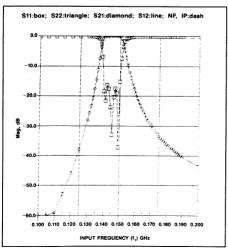
Figure 12. Calculated wideband response of example filter.
