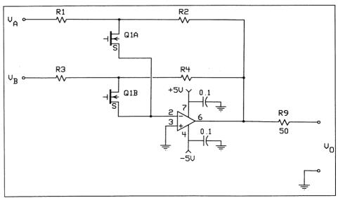
Figure 3. FETs in op amp feedback loop.
