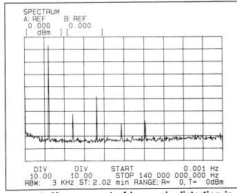
Figure 1. Measurement of harmonic distortion in a signal.
