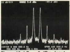
Figure 10. LO = -3 dBm, Input = +8.5 dBm, V\_BIAS = 2.2 V.
